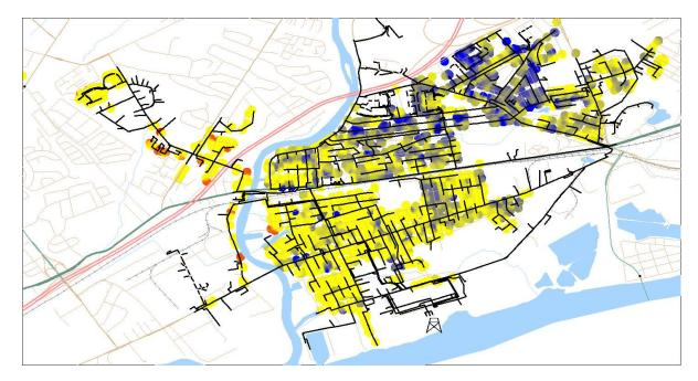
While the voltage profile is within the Tariff guidelines, voltages range from red/orange = >240v to blue/gray = < 240v
